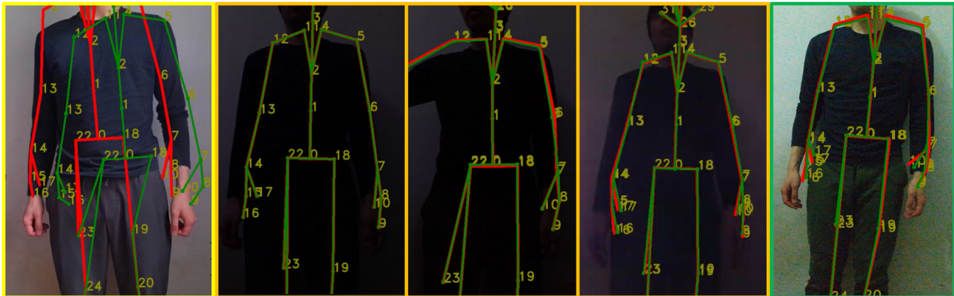
Figure 1: From left to right: (a) estimates from single (red) and weighted average (green) without transformation, (b) occlusion at subordinate #0, (c) occlusion at subordinate #1, (d) effect of direct light on master device, (e) final synchronized streams with offset due to parallax (red: single-device, green: 3-device system)
